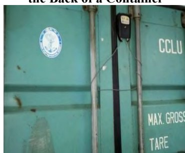
RECTS E-Seal Placed on the Back of a Container
