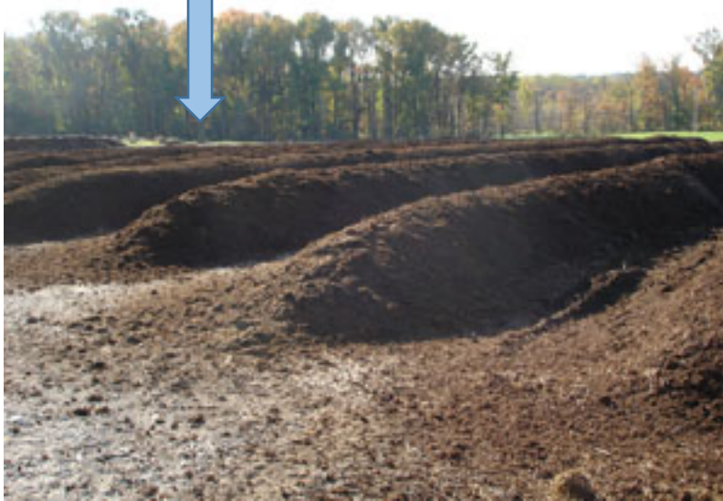
Production of uniform compost in windrows at a commercial composting facility.
