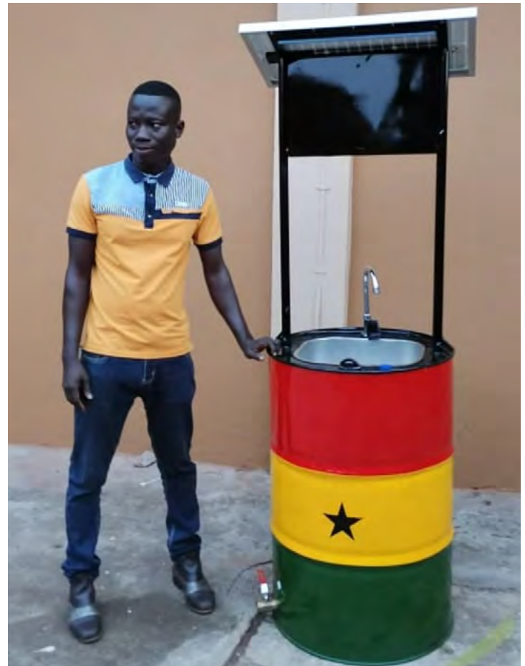
Photo: Solar powered hand washing device to encourage safe hand-washing practices, invented by a Ghanaian citizen
