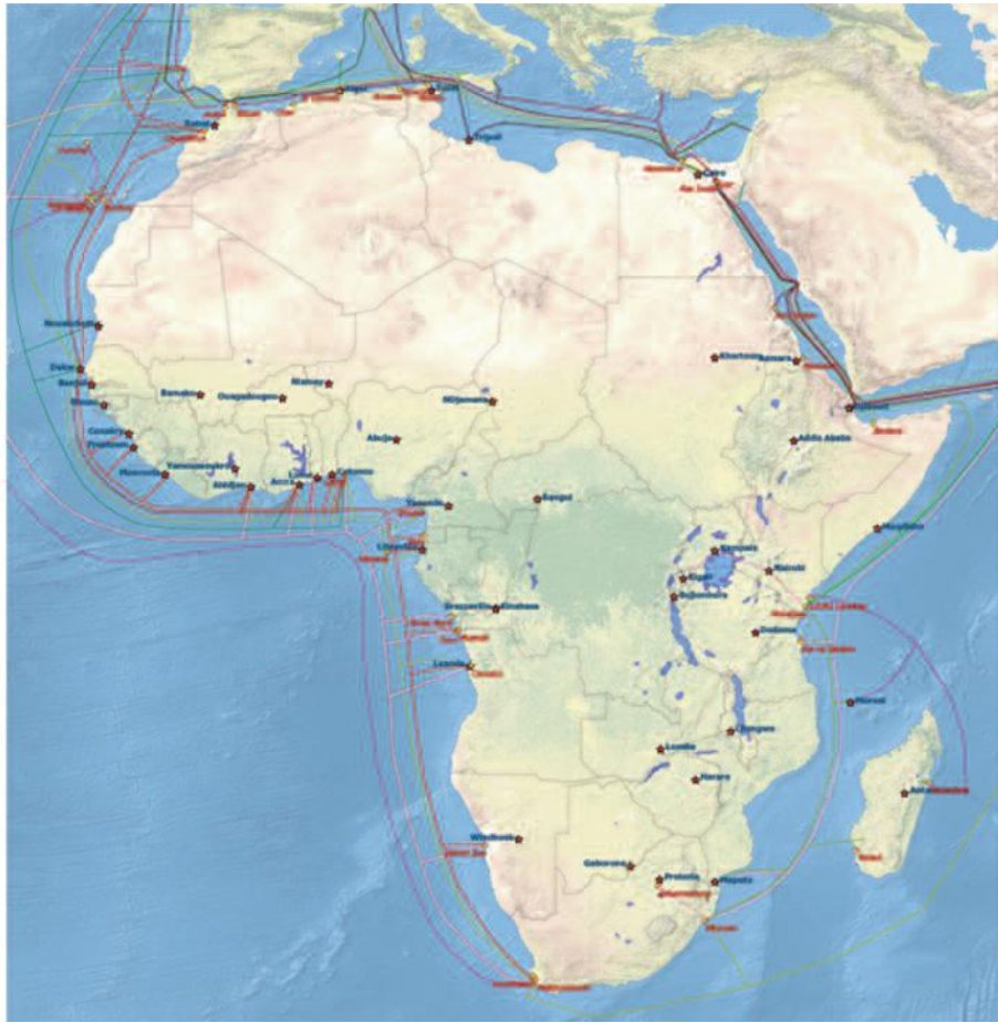
Figure 3a: Submarine cables
