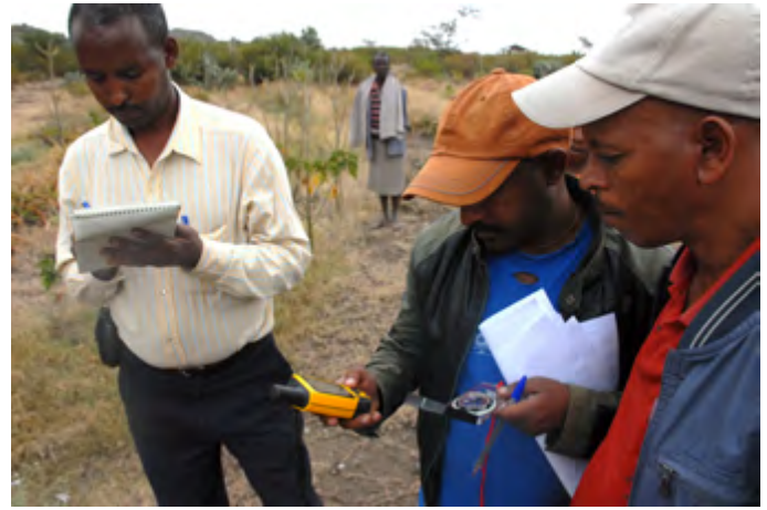
Figure 27. Members of the Tigray Team capture GPS and compass data while the scribe (at left) records the data in the logbook for a photo-point in the Tsega micro-watershed.
