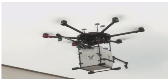
Figure 3: Drones were used to spray disinfectants on hard-to-reach areas. The drone carries around 15 litres of disinfectant and could cover a 1.5 km section in 15 minutes. This technique is very similar to what is done in the field
